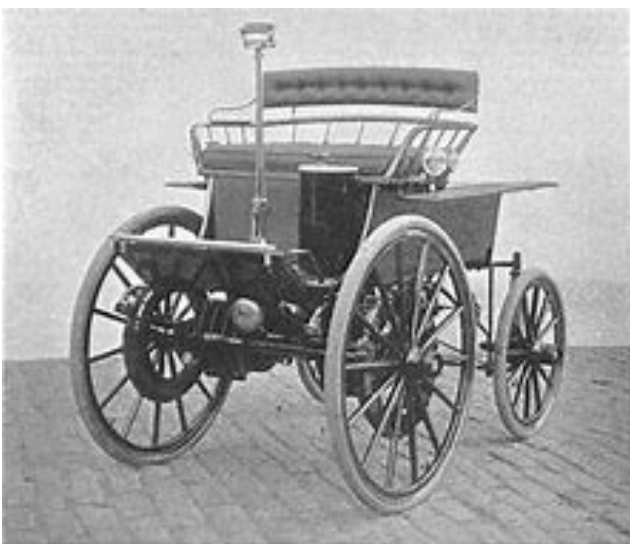
The Electrobat was one of the first electric automobiles. It was designed and built by mechanical engineer Henry G. Morris and chemist Pedro G. Salom in Philadelphia, Pennsylvania. Reorganised as the "Electric Vehicle Company", they patented their Electrobat automobile 31st August, 1894
